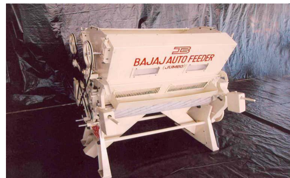
A photograph of improved Double Roller Gin with Auto Feeder / Lattice Feeder
