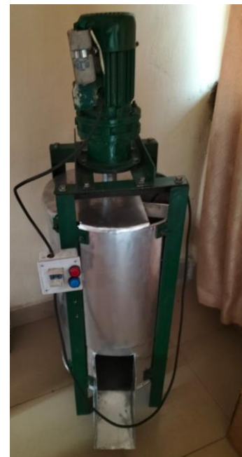
Fig. 3: Locally fabricated Palm Fruit Digester
