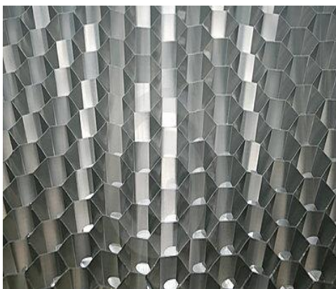
Fig 1 : The aluminium honey comb structure is shown below.
