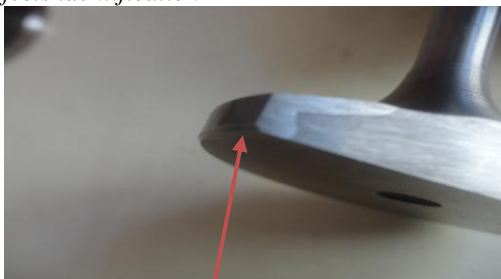
Fig (a) Stellite deposit overflow
