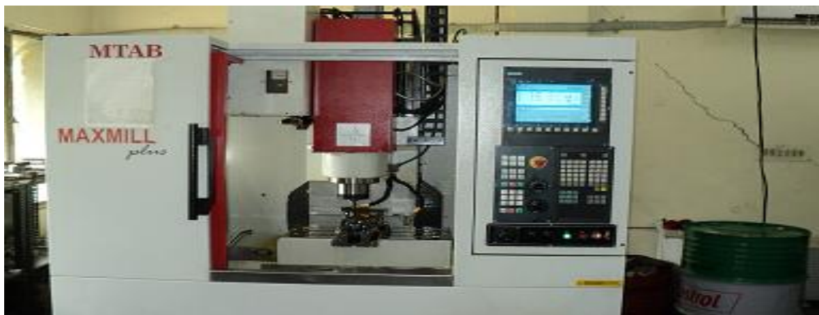
Fig.2: CNC vertical milling machine used for experiment Machine Model: MTAB MAX MILL PLUS
