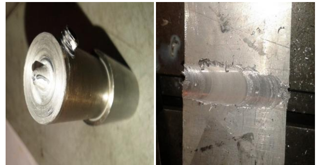
Fig.14 Tool after welding F.15 work piece after welding
