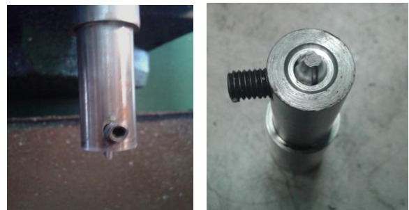
Fig. 7(f) Friction stir welding taper cylindrical tool with three flutes
