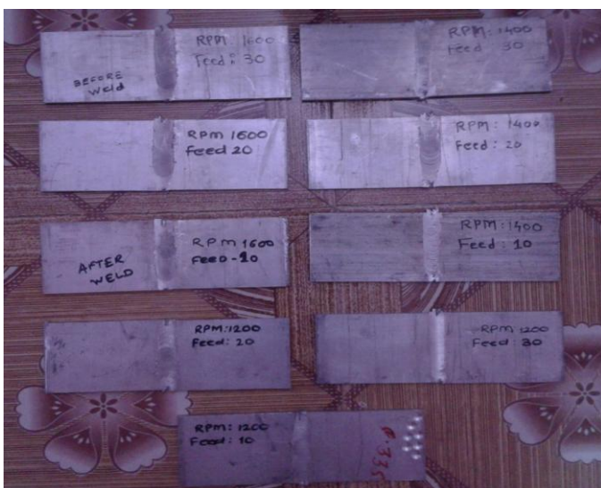
Fig.10 Work piece after friction stir welding
