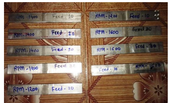
Fig.11 Tensile specimen before failure
