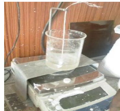
Fig. 3. Determination of density
