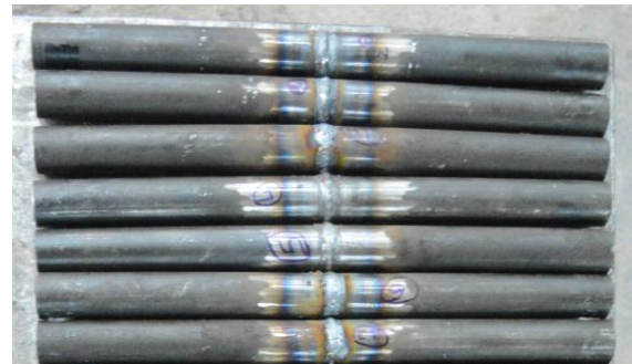
Fig. 3: Welded ASTM A106 Pipes
