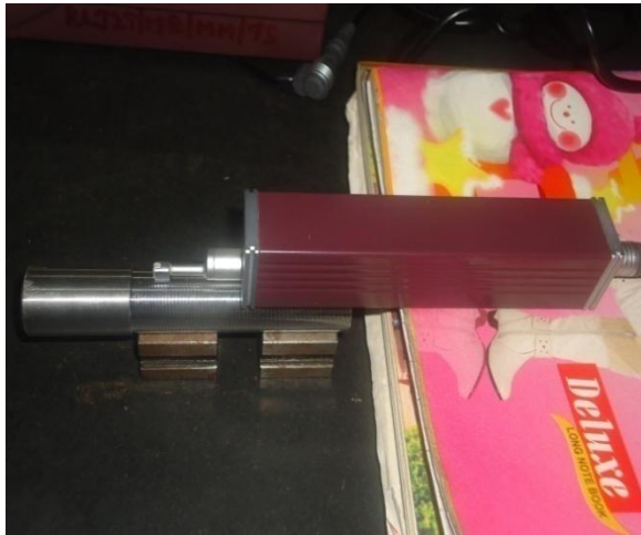
Figure 4: Profilometer which is used to measure Surface Roughness
