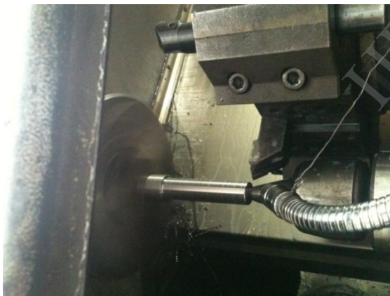
Figure 4.2 – Experimental Setup To Measure Hardness by Machining
