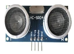
The amount of time during which the Echo pin stays high is measured by the MCU/MPU as it gives the information about the time taken for the wave to return back to the Sensor. Using this information the distance is measured as explained in the above heading.
