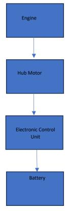
System proposes a solution by retrofitting existing scooters into hybrid electric which runs on IC engine. Here scooter with engine capacity of 125cc petrol IC engine is used. Also the rear wheel gets an electric hub motor. It becomes a conventional engine powering at the rear wheel and electric motor driving wheel.
