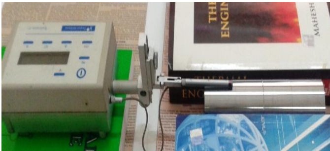
Fig.7. Taylor Hobson Surface roughness tester operation on workpiece (set up)
