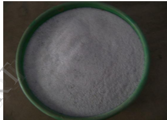
Fig. 2: glass powder passed through 300 micron sieve
