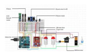
The circuit diagram for a vehicle that combines line following, obstacle avoidance, IR remote control, and Android application control involves connecting several components together to create a complex system. The Arduino board serves as the main controller, and it is connected to various shields and sensors, including the motor driver
