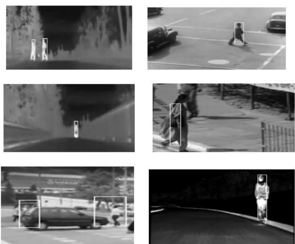
Fig.10: Videos used in verification, Pedestrians are detected by white boxes
