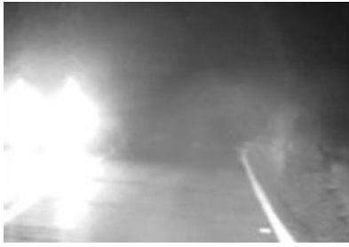
Fig.11: Missed detection due to external light source
