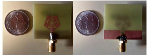
Figure 7: Patch and Ground plane layout of manufactured antenna
