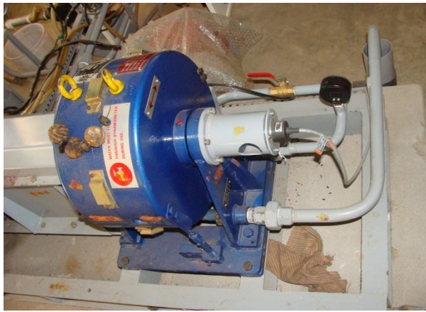
Fig.5. Eddy current dynamometer for loading
