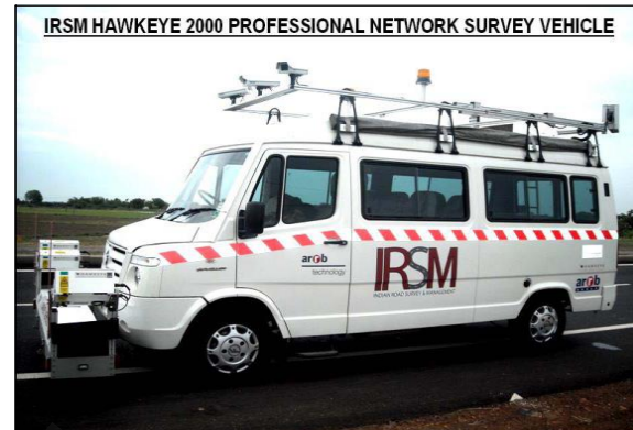
Figure 5.1. Showing ISRM Hawkeye 2000 Professional Network Survey Vehicle
