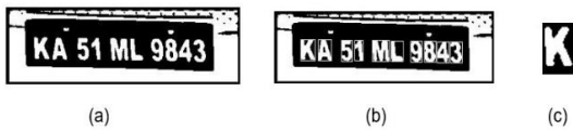
Fig 12. Post-Processing (a) Binarized image (b) Segmented Characters (c) Segmented character with median blur
