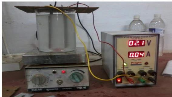
Plate-1: View of Experimental Set-Up (Iron Electrodes)
