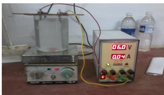
Plate-2: Pictorial View of Experimental Set-Up (Aluminium Electrodes)
