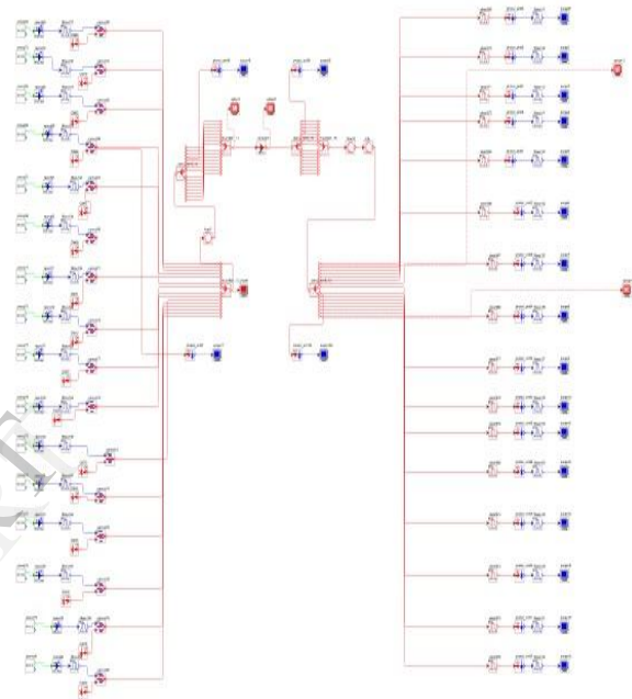
Fig. 2. Simulation model for a 16 channel DWDM Transmission system
