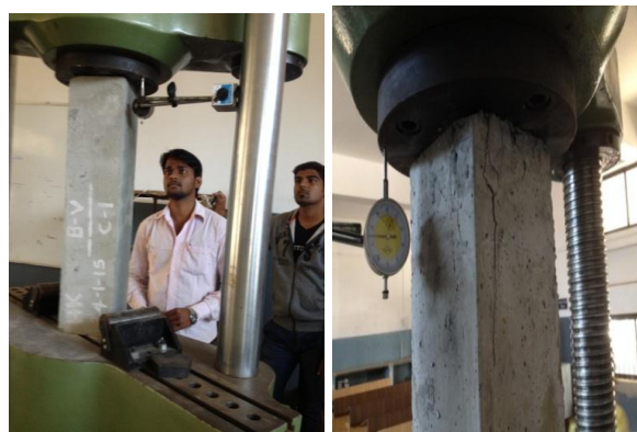
Fig 7 (a) – Experimental test setup and crack pattern.
