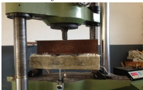
Fig 6 (a) Failed RC Beam wrapped with GFRP
