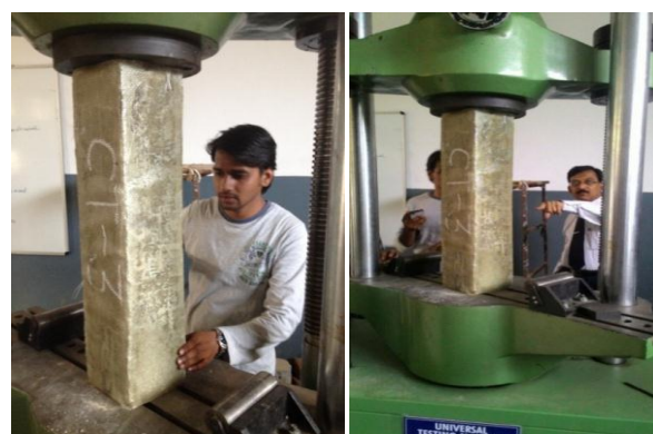
Fig 7(b) – Failed RC Column strengthened by GFRP.
