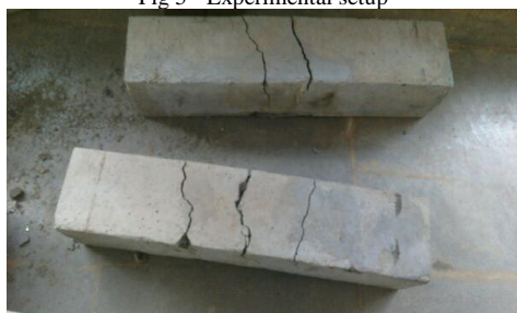
Fig 6 - Failed RC Beam
