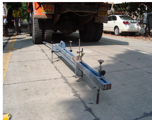
Figure 1: BBD Test on UWT in Progress
