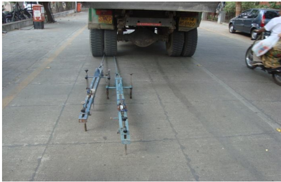
Fig.5: Two Benkelman Beam Used for LTE
