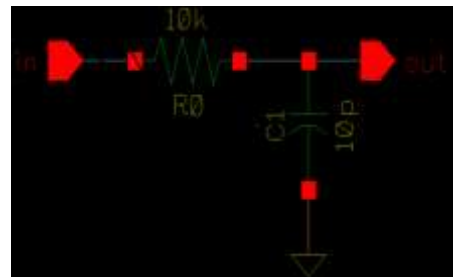
Figure (6): Low Pass Filter
