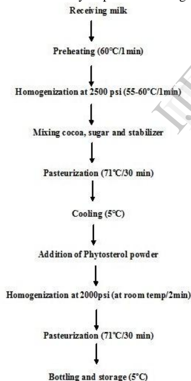
Figure 1. Methodology for the preparation of PS enriched low fat flavored milk
