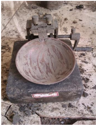
Fig.3 Liquid limit apparatus
