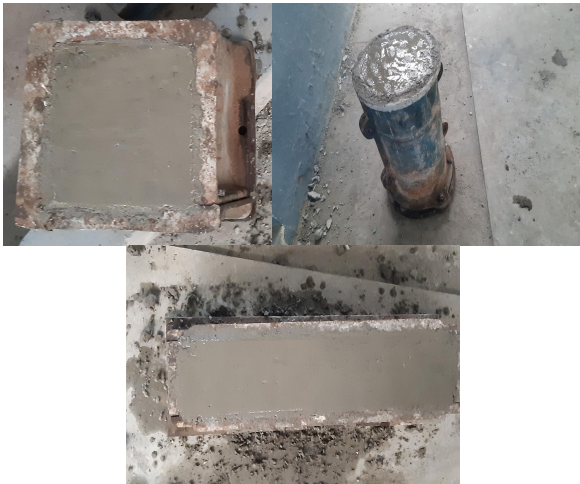
Figure 5: Casting of specimens
