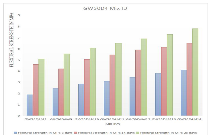
Figure 15 : Flexural strength test for Category GW50D4
