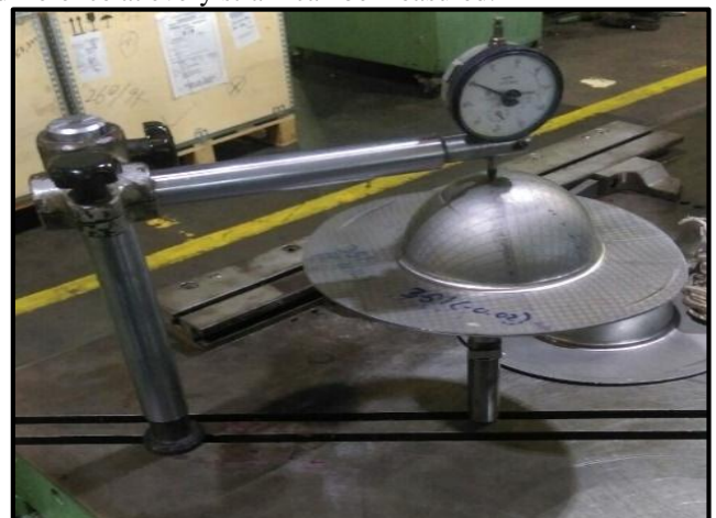
Fig 7. Thickness Measurement with Dial Indicator
