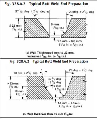
The end connections are aligned and temporarily secured with tack welds. After tack welding, a groove weld permanently joins the connections. This method is common for pipe sizes NPS 2" and larger, as aligning and welding smaller pipes can
