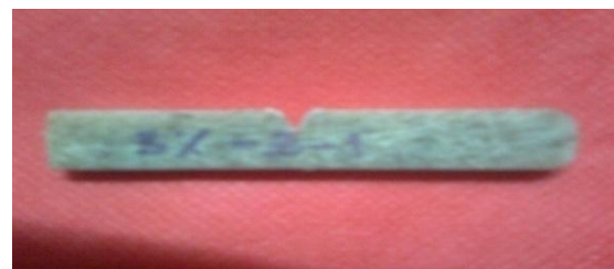
Fig.2.2. Specimen before impact test
