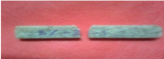
Fig.2.4. Specimen after impact test
