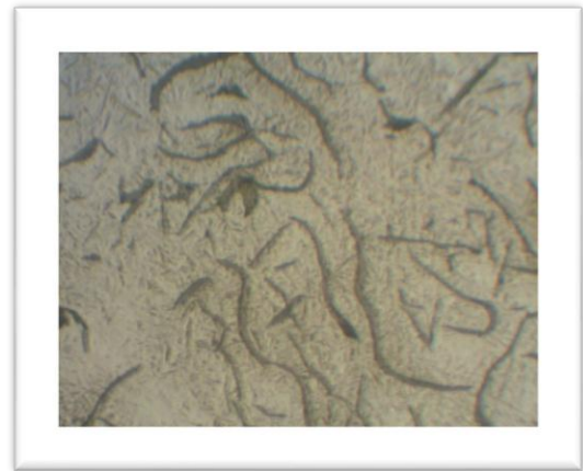
Fig 3 . Optical micro structure of Hardened Gray Cast Iron
