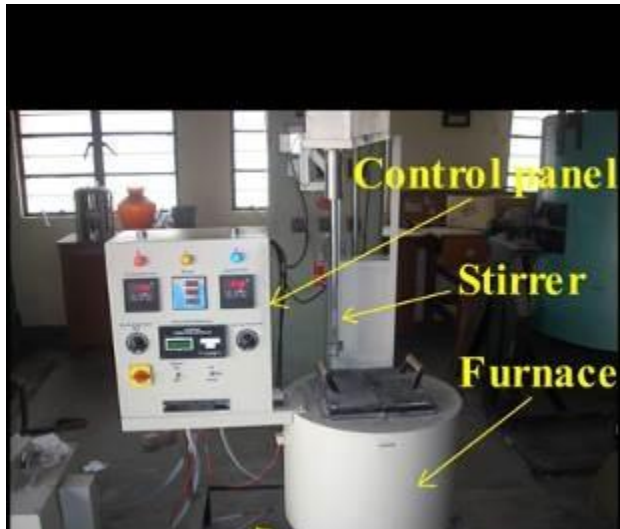
Fig. 1. Stir casting facility.
