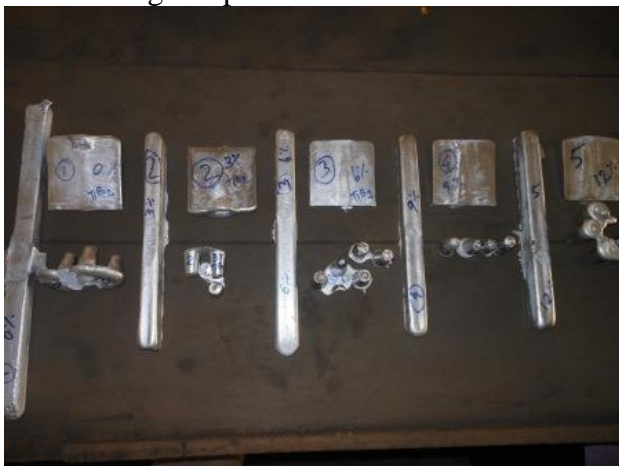
Fig 2: Casting samples with different compositions
