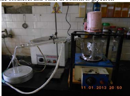
Fig.1. Esterification and Transesterification Setup
