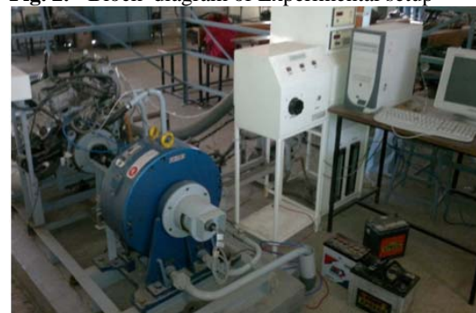
Fig. 3. - Experimental set up of SI engine
