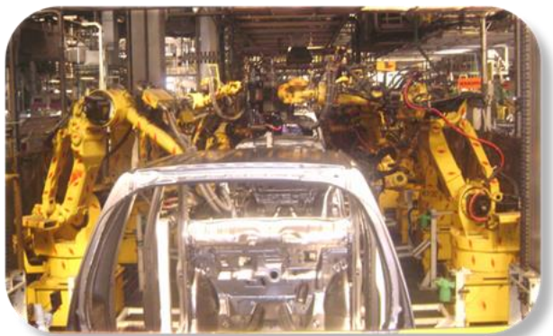
Figure 3: Pictorial view of Multi robot spot welding process
