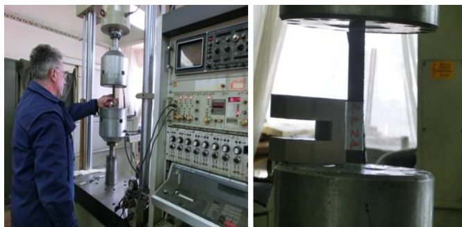
Fig.6. Tensile test on universal testing machine.
