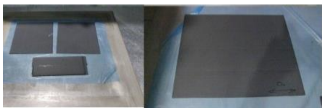
Fig. 4. Finished composite parts from vacuum bagging.
