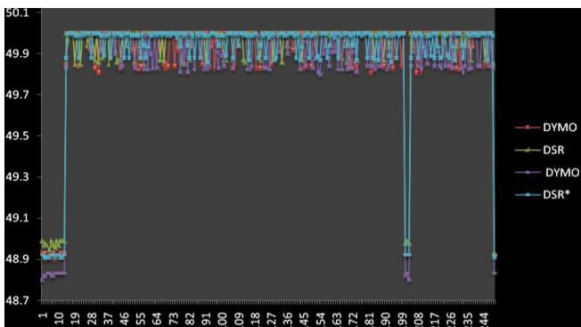
Fig. 35 Comparison of Residual Battery Capacity of DSR and DYMO using CBR and Traffic-Gen.
