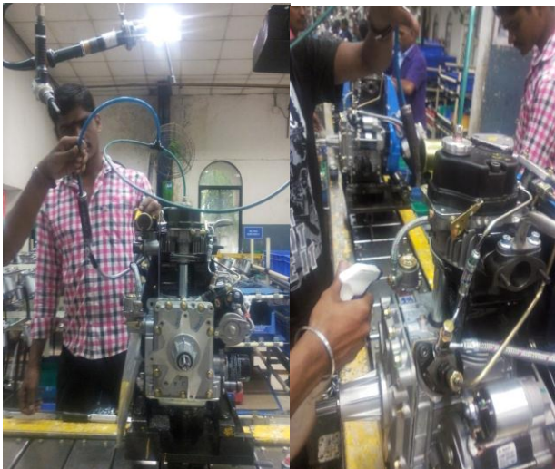
Figure 2.4 Leakage findings in the engine whether engine is Ok or Not Ok
