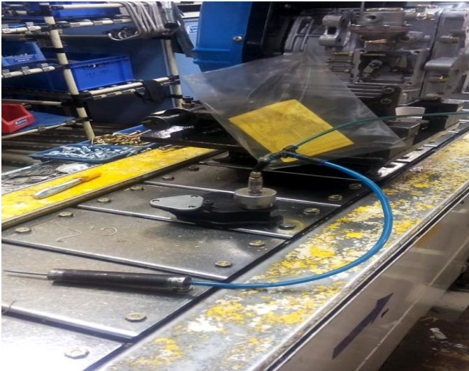
Figure 2.3 Air supply through rocker cover & overflow pipe
