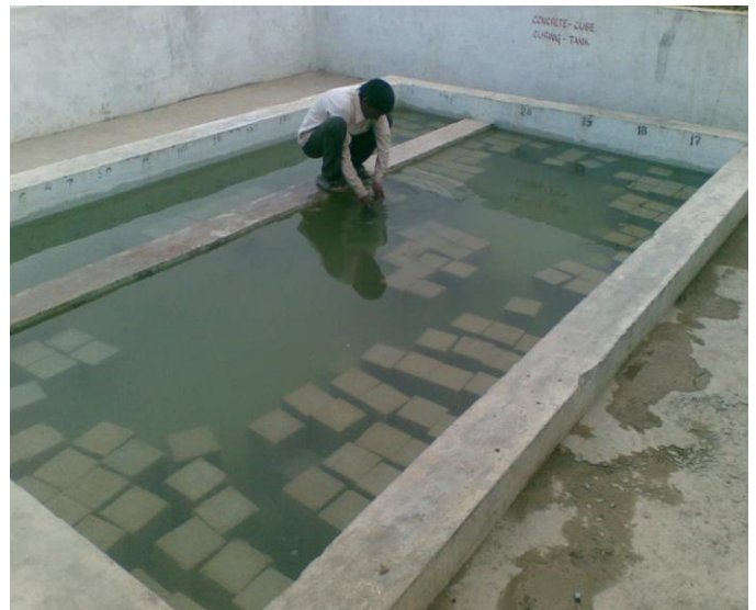
Figure – 3: CC cubes under water
