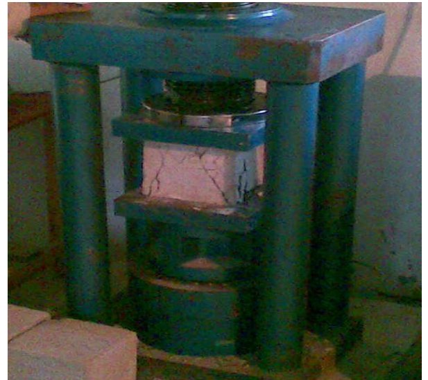
Figure – 5: CC cube under Compression
