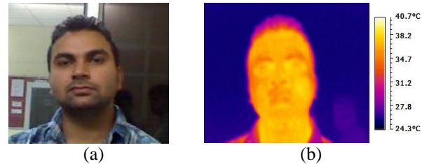
Fig. 1 (a) Visual image of human face where each pixel shows natural colour (b) Thermogram of human face where value of each pixel is temperature dependent.
