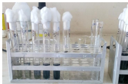
Fig.IV. Standard Protein assay by Folin Lowry's method crude protease enzyme for quantitative estimation of Protease
