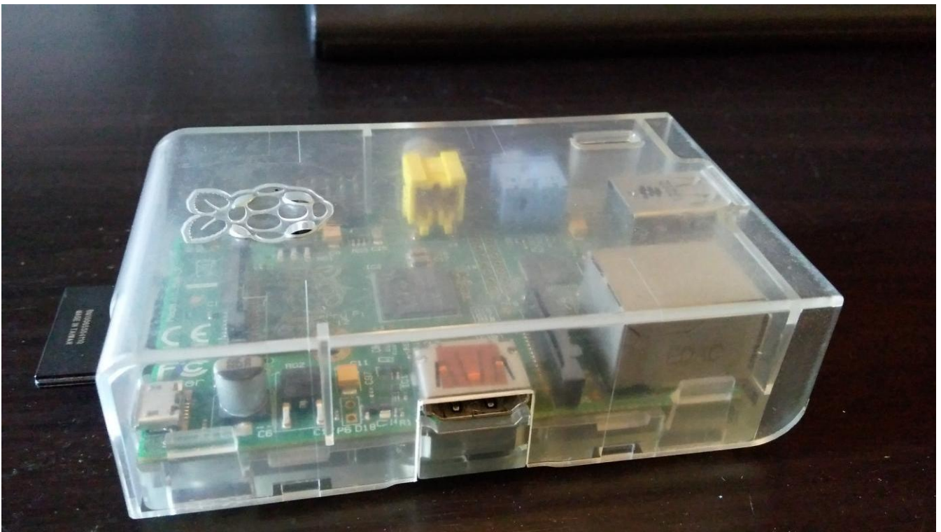
Fig. 1. Raspberry Pi enclosed in a clear plastic case with the SD card on the left.
