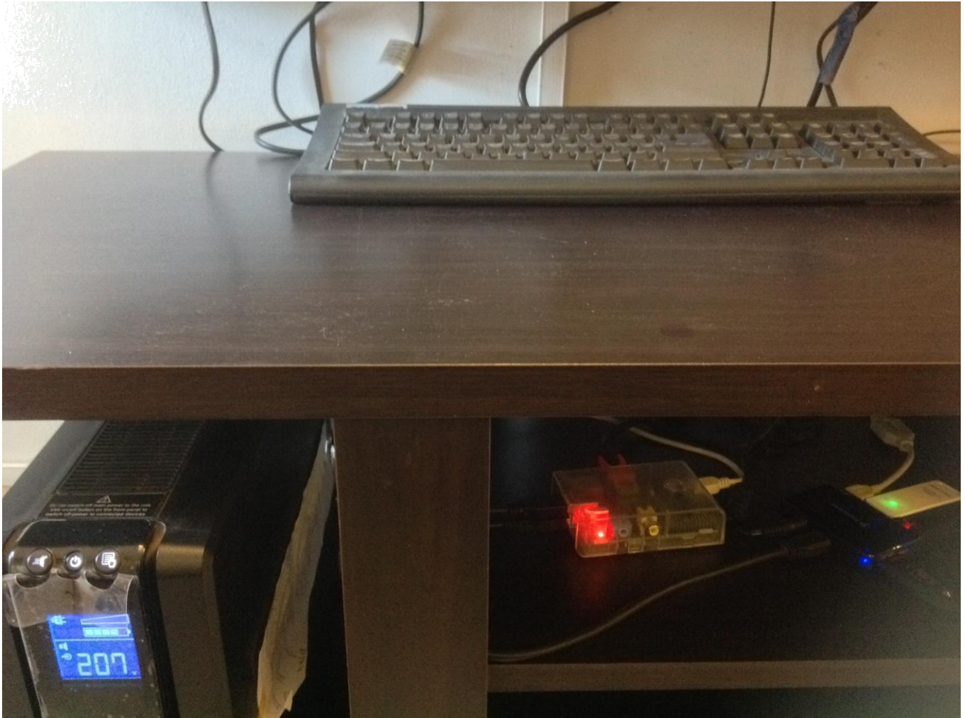
Fig. 2. Picture showing Raspberry Pi attached to smart UPS, and via a USB hub to a pen drive, Wi-Fi dongle, keyboard, mouse and TV (TV not shown).
