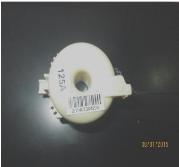
Fig. 3. Input image of a current transformer
