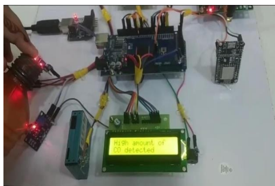
Fig.12.1 High Amount of CO detected and Displayed on LCD
