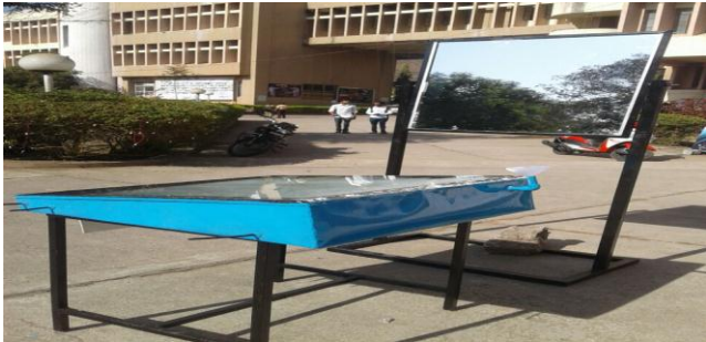
Fig:-.4.1 Regenerative Solar Still With Concentrator
