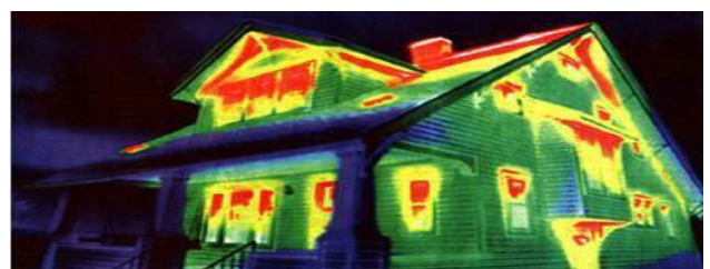
Fig.7. IR testing for leakage in building
