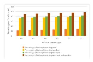
The above graphs is between Adsorbent volume percentage vs Percentage of Adsorption. In this Volume percentage is in X-axis and Percentage of Cr ions adsorbed is in Y-axis. This graphs clearly shows that the percentage of adsorption
