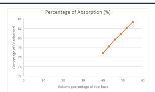
The above group is between Volume percentage of rice husk vs Percentage of Adsorption. In this Volume percentage of rice husk is in X-axis and Percentage of Cr ions adsorbed is in Y-axis. This graph clearly shows that the percentage of adsorption increases with increase in the adsorption volume percentage of rice husk. The rice husk adsorbs 83.34% of Cr about ions industrial waste water.
