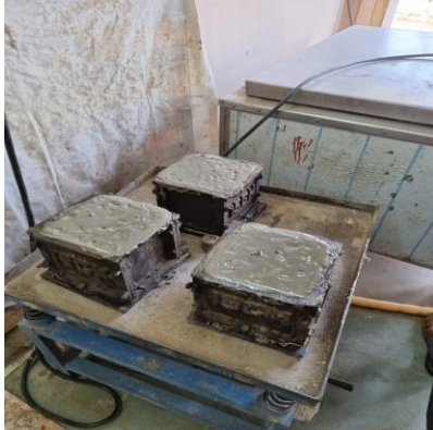
Fig 2: Casting of cubes
