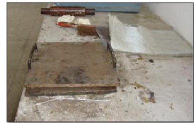
Set-up of hand lay-up process
