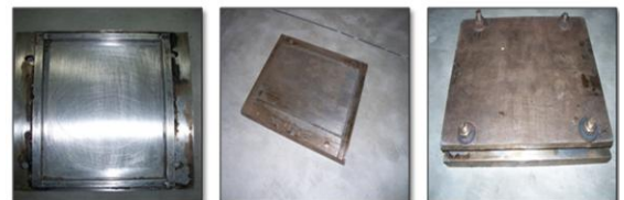
Fabricated steel mould cavity for the manufacturing of thermoplastic based natural fiber composites
