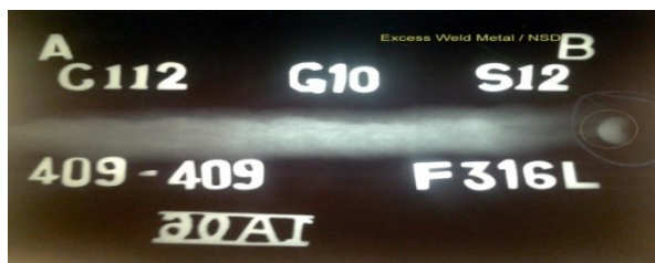
Fig. 3. Copies of X-ray radiographic film for sample no-4
